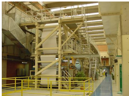
PC2 coater which is going to add more dryers
