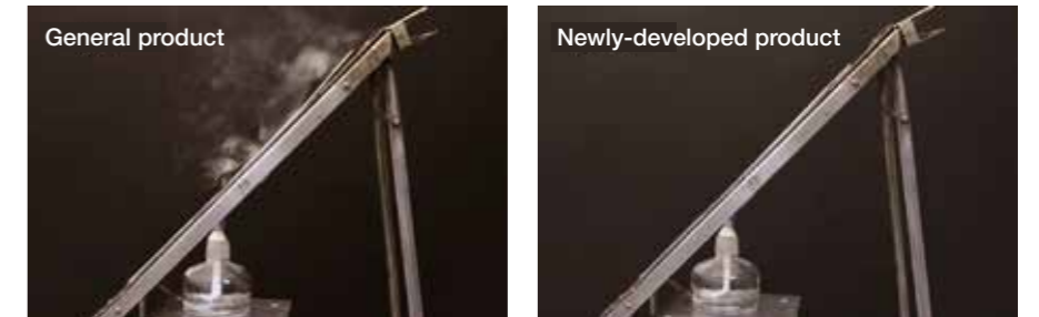
Smoke test with heating from alcohol lamp
