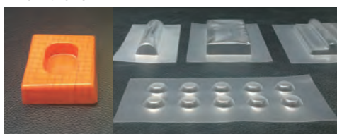
Stretched film with high flexibility and processibility
