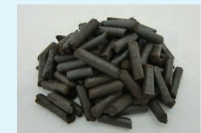
Black pellets (biomass-fuel wood pellets that are semi-carbonized)
