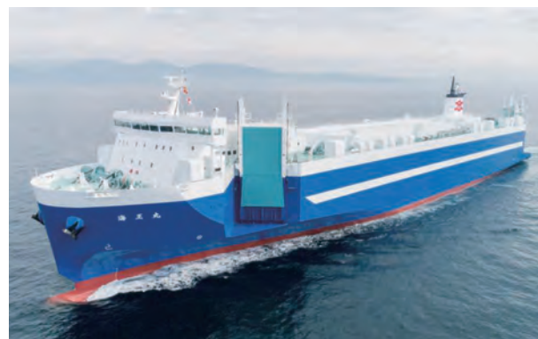
A roll-on roll-off (RORO) ship that can transport vehicles carrying goods
