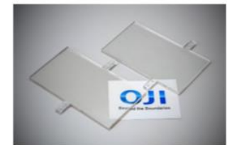
Polycarbonate composite using transparent CNF sheets
