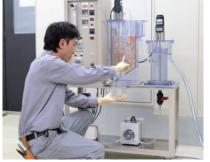
Laboratory testing apparatus for biological treatment
