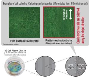
Flat regions and substrate pillars are interleaved in parallel stripes.
