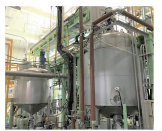
Testing plant for enzymatic degradation and fermentation
