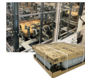
The packaging tray and auto-assemble machinery for large commercial-use air conditioner developed together with Daikin Industries, Ltd.
