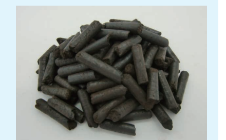
Black pellets (biomass-fuel wood pellets that are semi-carbonized)
